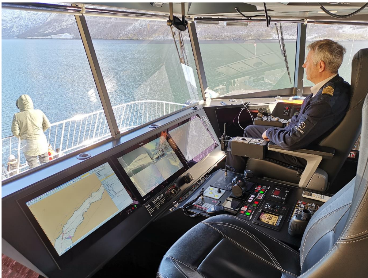
Photo 5. The energy and propulsion system on "Future of The Fjords" is highly automated. Monitoring, control and possible override is performed from the steering position on the bridge. Photo: Lars Haugnes
