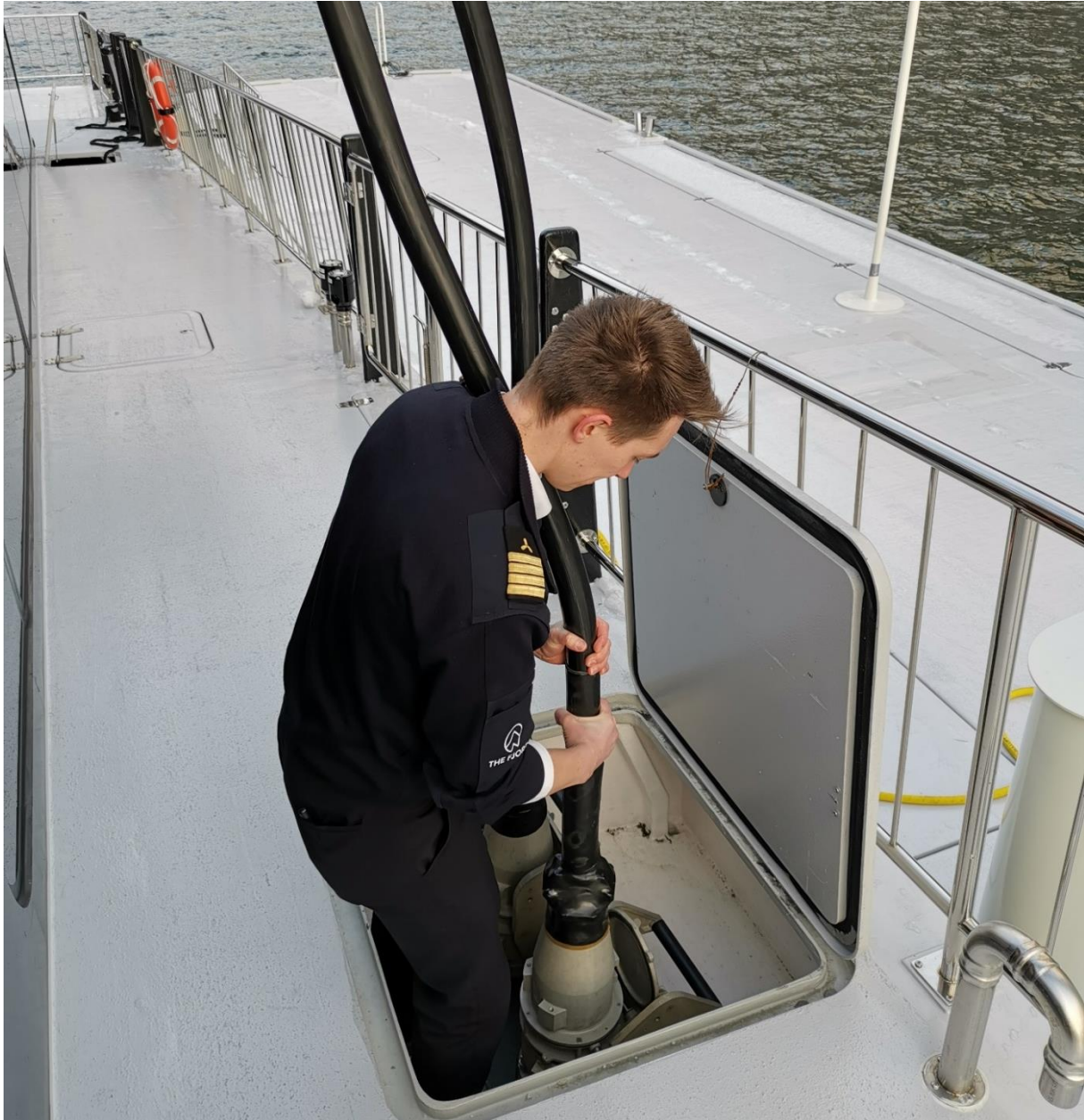
Photo 4. Connection of a charging plug to "Future of The Fjords". Two plugs are used to charge the battery packs. Each plug can charge with 1.2 MW power. Photo: Severin Synnevåg
